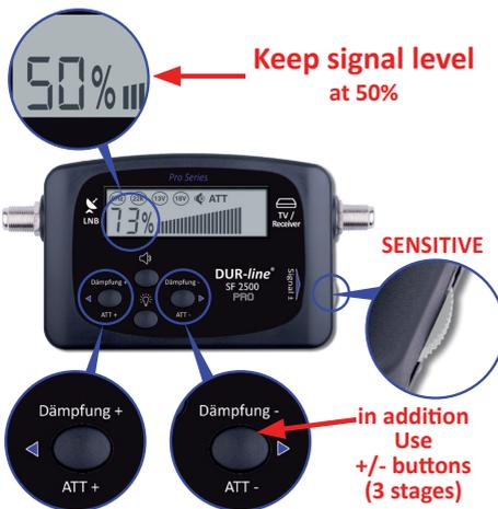
Keep the signal level display region at approx 50% by reducing or increasing the attenuation. An increase or decrease in the level can thus be identified. If attenuation is activated, “ATT” appears on the display.
